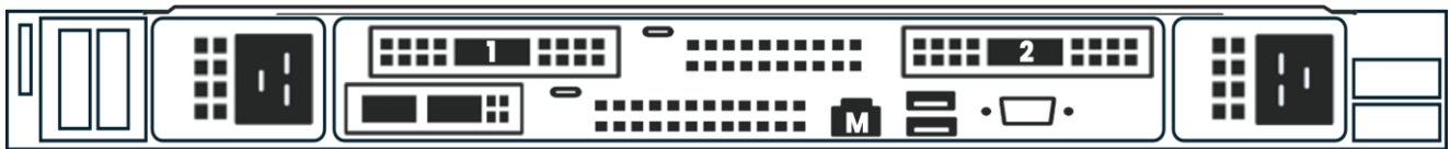
Figure 9. Recommended WEKA storage server network port connections.
