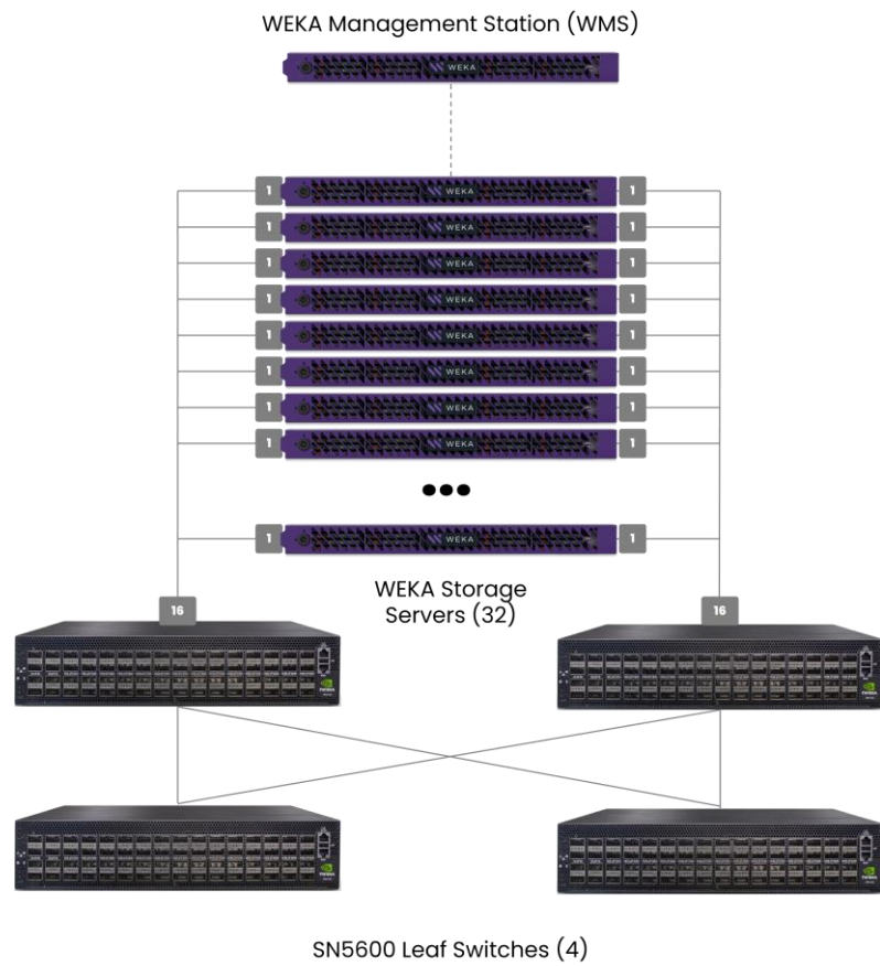
Figure 13. WEKApod reference architecture for NCP deployments with 1,023 HGX servers.
