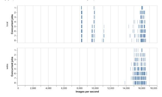
The results illustrate that the performance of the WEKA appliance is reliably around 16k images/sec, and in line with the best performance we have observed using local NVMe.
