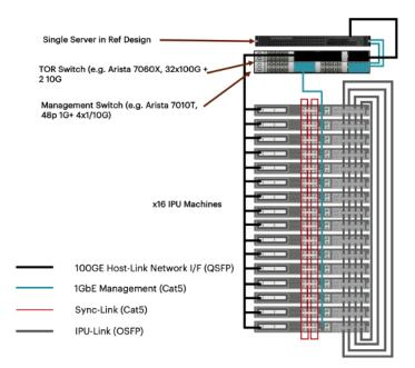
The IPU-Machine has a flexible, modular design, so you can start with one and scale to thousands. IPU-Machines can work as standalone systems or can be interconnected in racks. Individual IPU Pod racks can then be interconnected with other Pods using the 2.8Tbps high-bandwidth, near-zero latency IPU-Fabric™ interconnect architecture, to grow to supercomputing scale.
