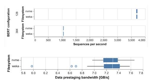
These results show that the performances of the local and WEKA.IO filesystems are comparable. The average bandwidth for each of the two filesystems is just above 7.3GB/s, with a similar distribution around this average. The WEKA.IO results show some outliers (shown as circles in the plot) where the performance dips to around 20% below the average.
