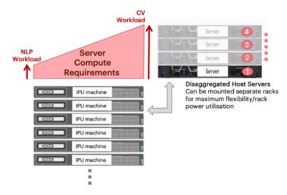
For example, NLP models require very little server CPU interaction and utilization, whereas CNN-based workloads such as CV require a larger proportion of scalar computing and would benefit from more server CPU being involved. The system can be tailored for the workload.
