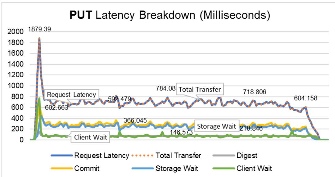
Figure 10. IBM COS upload PUT latencies.
