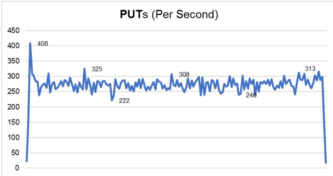
Figure 9. IBM COS upload PUT operations.
