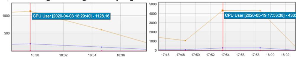
Figure 3. IBM COS 4105 Accesser GET CPU impacts, HTTP (Left) vs. HTTPS (Right).
