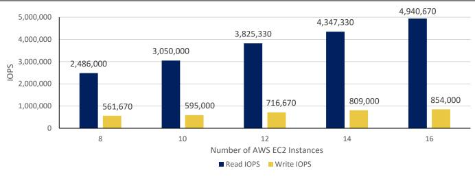
Figure 9. WekaIO Performance Scaling on AWS—IOPS
