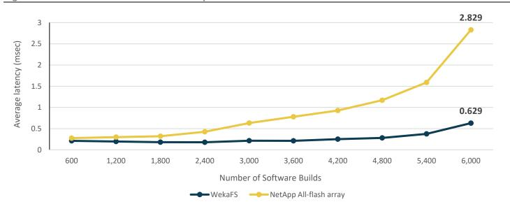
Figure 5. SPEC SFS 2014 Software Build Response Time Curve
